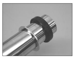
6. Use PV-49494 to install oil seal until seated. Be sure top edge of seal is past (below) retaining ring groove.
