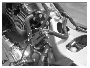
16. Disconnect diagnostic connector (M) and push harness and grommet (N) out of inner saddlebag to allow harness removal.
