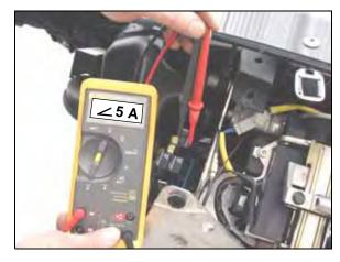
6. Inspect fuel pump circuit wiring or replace fuel pump if current draw exceeds specification.
