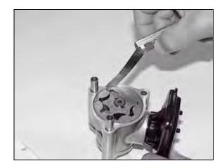
Measure the oil pump end clearance with a feeler gauge at point "A". Lubrication side of pump is shown below. Cooling side is measured in the same manner.
