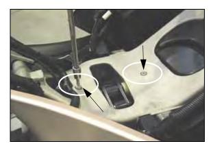
9. Drive pivot pin (C) from the <u>backside</u> forward, until clear of the suspension rocker arm. Leave driver in place.
