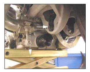
14. Continue to lower the motorcycle with the platform jack until the lower shock pushrod eyelet is aligned with the swingarm. Install bolt with nut on the inside. Torque the nut to 81.4 Nm (60 lb-ft).
