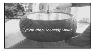
11. Pull bearing in to right side of wheel until seated against spacer.
