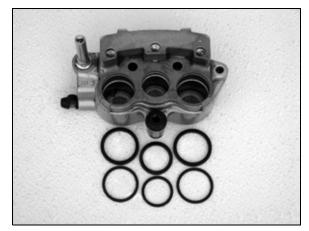
Clean all parts thoroughly with isopropyl alcohol. Be sure the seal bores are clean, removing all traces of dirt or dried brake fluid.
