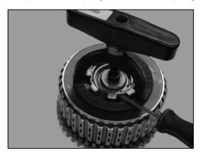
4. Remove retaining ring seat (B) (stepped washer).
