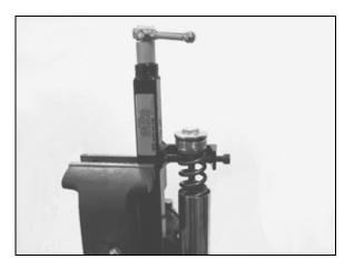
10. Hold nut and remove fork cap (F) from cartridge shaft.
