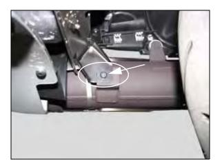
6. Loosen both the muffler clamp and the crossover pipe clamp on the left side, and the muffler clamp and head pipe bolt (near the crossover pipe) on the right side.
