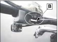
Front brake micro switch located on front brake lever perch
