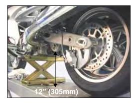
8. Remove the drive belt-side wheel spacer and disengage drive belt from rear sprocket.
