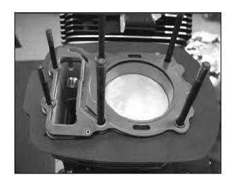
4. Clean gasket surface on cylinder head and set cylinder head in place on cylinder.
