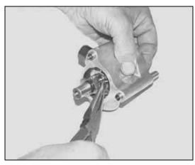
12. Secure pump base in a soft jaw vise. Apply Victory engine oil to threads of cooling pressure relief valve and install into pump base. The cooling relief valve has a longer hexagonal portion than the lubrication relief valve. Torque to 27 Nm (20 lb-ft).
