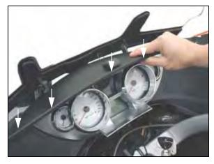
6. Install visor screws and torque to 4.0 Nm (36 lb-in).
