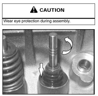
1. Lubricate valve stems with assembly lube.
