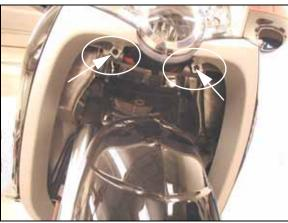
6. Remove the screws at the front and rear of each outer leg fairing.
