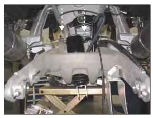
11. Remove shock, rocker arm, and pushrod as an assembly when clear of the frame.
