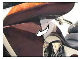
2. Remove (2) T-20 Torx screws that attach deflector to pivot hub.
