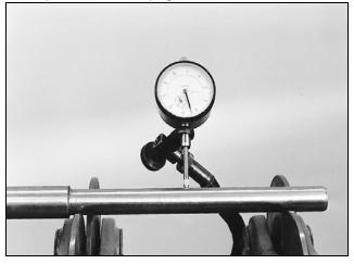
2. Replace axle if it fails inspection. Do not attempt to straighten a bent axle.
