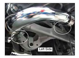
Hook slot (A) of Exhaust Muffler Wrench PV-49946 on muffler bracket (B) as shown below. Pull handle of tool to rotate muffler until studs (C) are clear of mounting slots on inner saddlebag.
