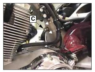
10. Remove driver while guiding bottom shock mount into opening in swingarm with pushrod along side.
