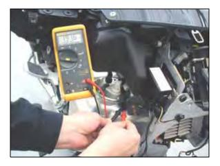
4. Attach the meter leads to pin C and pin D of the 4- pin connector out of the fuel pump. Estimate the fuel level in the tank and compare resistance reading to the table below.
