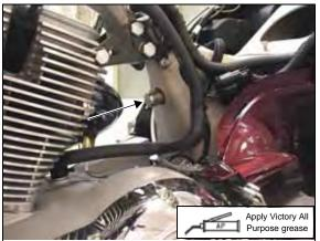
3. Drop the shock assembly down through opening in swingarm with pressure hose routed between pushrod and vent hose. Raise shock into position.
