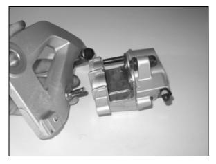
Remove caliper pistons. Keep pistons in order for installation in their respective bores.
