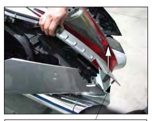
Lift high enough to release peg that secures rear of lower access panel.
