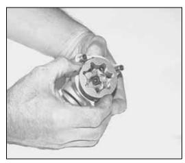
11. Push shaft toward lubrication side and hold in place. Install pin for lubrication rotor. Lubricate both gerotors with oil.
