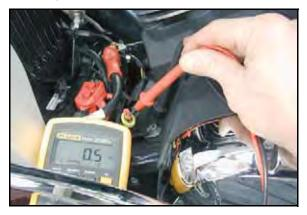
• Release clutch lever, meter should display a higher resistance in the range of 2K - 9K (2000 -  $9000\Omega$ ).
