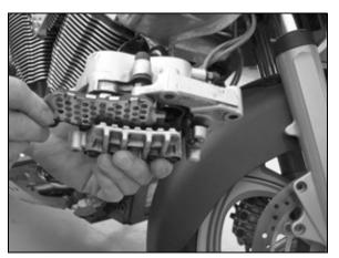
Remove the spring plate and pad retainer from the caliper; note direction of plate and retainer for assembly.
