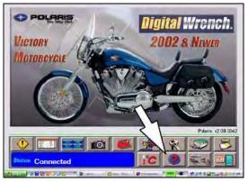
6. <u>COMMUNICATION PROBLEMS</u>: If you have had problems communicating with a vehicle while performing diagnostic functions, do not attempt reprogramming until the cause has been identified and fixed. Check all connections, and be sure battery voltage is as specified in Step 1.
