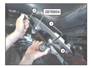
6. To INCREASE pressure, install the gauge select the desired pressure from the chart as described in steps 1-4 above. Pump the handle (3) until pressure increases to the desired amount, then remove the hose and install the cap.
