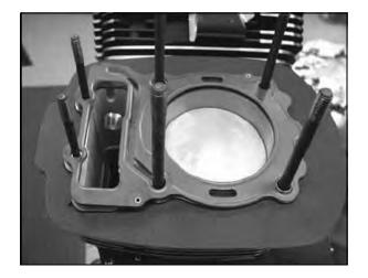
4. Install cylinder head onto cylinder.
