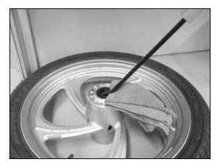
4. Remove snap ring from disc side.
