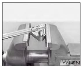
13. Install oil jet to oil pump base. Torque to 13 Nm (115 lb-in)
