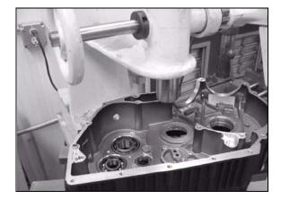
2. Press balance shaft bearing from the primary side using an arbor press (B).
