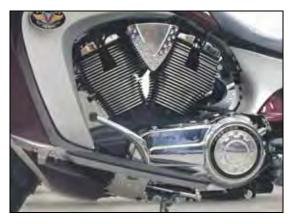
2. Lubricate the shift pedal pivot bushing with Victory All Purpose Grease P/N 2872187 (page 9.6).
