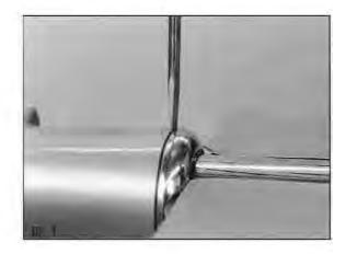
Remove damper rod bolt and sealing washer. III. 2.
